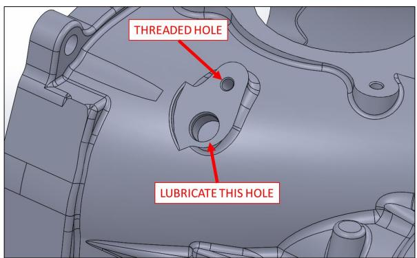
\*\*NOTE: The sensor's mounting fastener comes from the factory with a dry blue locking compound. If this sensor has been removed several times, the locking compound may have lost its ability to retain itself in the threaded hole. A small amount of blue liquid locking compound can be utilized to aid in the sensor's ability to resist loosening on the supercharger.\*\*
